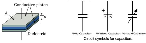
Capacitors can be used when a rapid discharge of energy is required. (Batteries supply charge at a much slower rate). For this reason they are the basic component in camera flashes, Tasers and heart defibrillators. A defibrillator is a device that administers a controlled electric shock to a person experiencing cardiac arrest.
