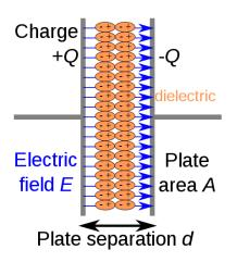
Schematic of a parallel plate capacitor with a dielectric spacer. Two plates each with area A are separated by a distance d. When charge is established on the plates, an electric field exists in the region between the plates. The dielectric material becomes polarised due to the charge displacement and increases the capacitance.
